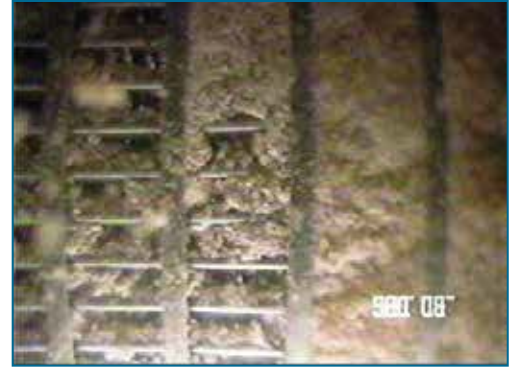
FIGURE 39. Scale formation on a well screen. (Source: Gary Hix)
