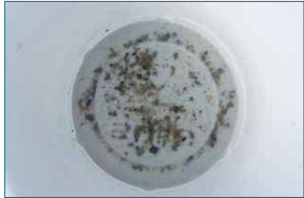
FIGURE 36. Sand accumulated on the screen of an irrigation system. (Source: Mike Prestigiacom)
