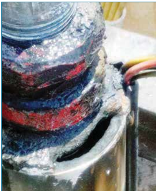
FIGURE 35. Stray electrical currents formed a hole in this submersible pump. Water was forced through the hole in the bottom of the pump, causing the well screen to collapse and the well system to fail. (Source: Mike Prestigiacom)
